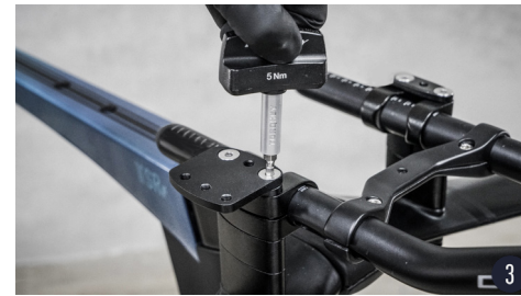
Use the No. 5 hex wrench and the No. 4 torque wrench to tighten the screws by 5Nm.
