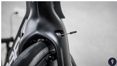
Please pull out the excess brake line out of the front brake cover to make sure the braking efficiency.
