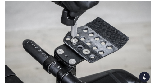
Screw the arm pad plates on the corresponding spot on both sides by 5Nm.
