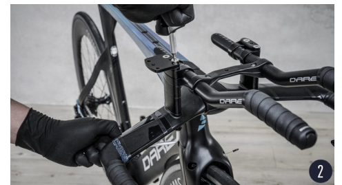
Loosen bolts and screws then remove the arm pad mounts [D7, D8]. Add the extended plates [D5, D6] (Letters facing downwards, R on the right hand side and L on the left hand side). Tighten the bolts and screws again.
