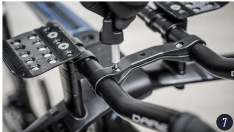
Adjust extension bars and tighten the mount bridge [C1].
